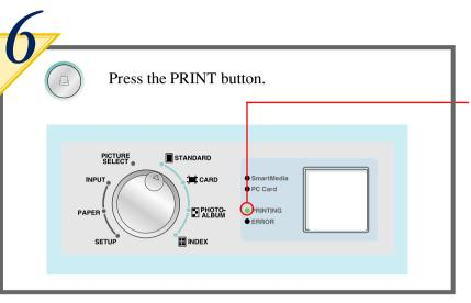
The lamp flashes when the PRINT button is pressed after which printing begins.
